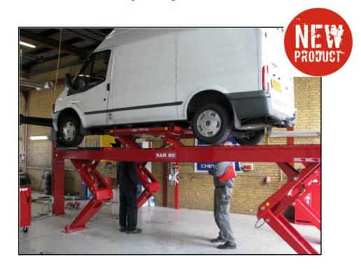
A new **Auxiliary Lifting Table** engineered for KAR 60 lift for **long wheel base commercial vans**.
